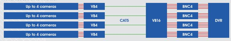
Ideal for multiple individual cameras back to a single 16 channel balun rack unit. Clean installs for CAT5 to convert to BNC. 3p = 19 gauage
