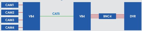
Ideal for individual runs (homerun) to each camera. Be sure remaining pairs provide adequate power, unless using remote power. 3p = 19 gauge
